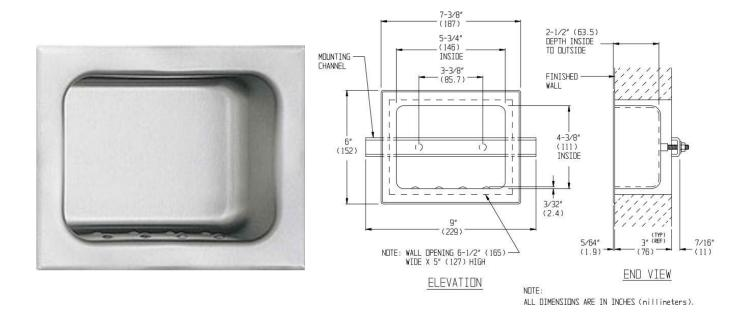
Model WA140 is a recess mounted soap dish. Manufactured from grade 304 stainless steel with a satin finish. This model is recessed into the wall with a front mounting flange on the front. The soap dish has two nuts welded on the back for rear mounting. The soap dish itself has raised dimples on the base to elevate the soap allowing the air to circulate.
